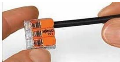
Lower the lever to close the clamping unit. Flip the housing over to visually verify that the exposed wire is contacting the metal clamp.
