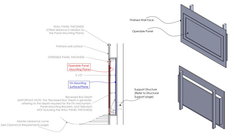
Clearance Gap around panel: As the operable panel flips around it will enter the recessed opening as it approaches the TV viewing position. Therefore, the recessed opening must be larger than the operable panel. (see clearance considerations sheet)
