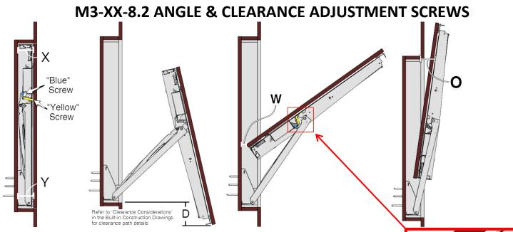
Each arm has two independent adjustment screws. Yellow, adjusts the closed position angle and Blue adjusts the open position angle as well as the clearance. Note: The true results of your adjustment will not be seen until the mount is operated once after the adjustment is made.
