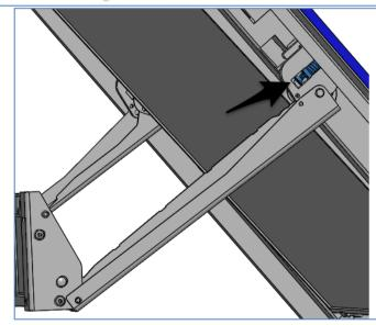
SPRING 2, located in ONE ARM ONLY, slows the mount as it approaches the TV Viewing Position. It can also be used to adjust the viewing angle of the TV.
