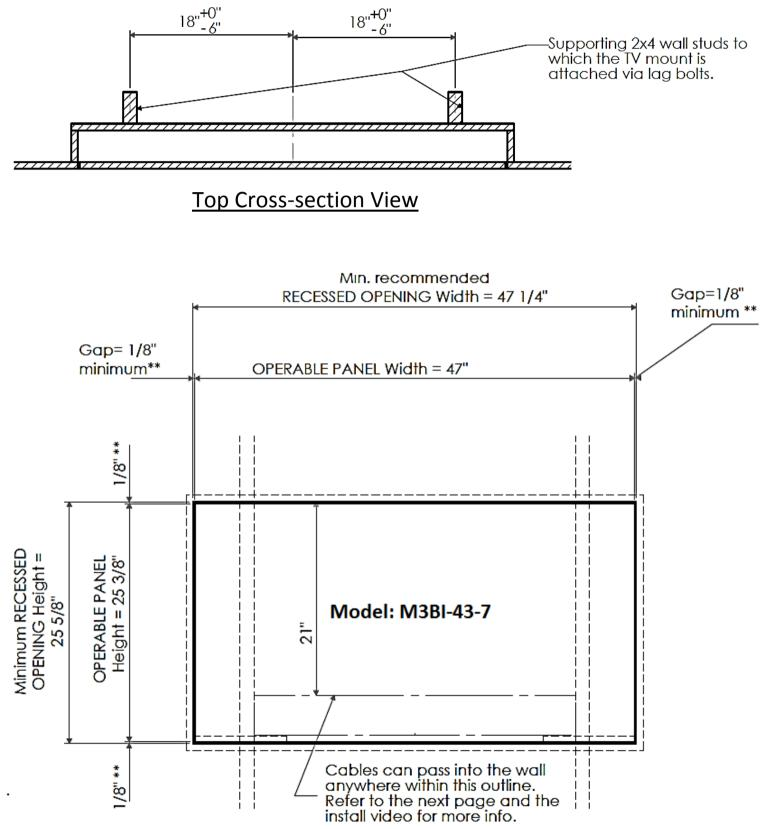
\*\*Minimum Gap: As the operable panel flips around it will exit and re-enter the recessed opening. Therefore, the recessed opening must be larger than the operable panel. We recommend a minimum 1/8" gap on the sides.
