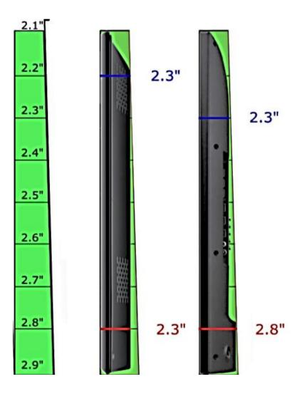
Place TV inside the mount with the screen facing the wall and upside-down
