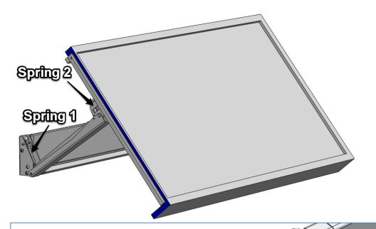
SPRING 1, at the base of each arm, controls the speed at which the Picture Frame approaches the wall when closing to the hidden position
