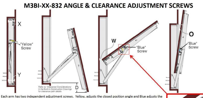
Each arm has two independent adjustment screws. Yellow, adjusts the closed position angle and Blue adjusts the open position angle as well as the clearance. Note: The true results of your adjustment will not be seen until the mount is operated once after the adjustment is made. Feel free to contact us to assist with fine tuning these and other adjustments. We have excelent tech support! Call or text Mark 208-919-5969.
