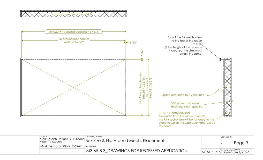
Clearance Gap around panel: As the operable panel flips around it will enter the recessed opening as it approaches the TV viewing position. Therefore, the recessed opening must be larger than the operable panel. (see clearance considerations sheet)
