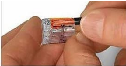
Strip the wire to 7/16" (11mm) (refer to strip length guide printed on the side of the connector)
